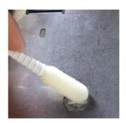
You should clean sensor prism (transparent plastic parts) as well as the sensors on the cover plates, which are easy to recognise. These are small recesses, which are arranged in pairs at intervals of about 1cm to each other.
