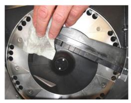
Please wipe the solved dirt desposits from the front sensor, the coin run and the coin forward tray and its triangles with the dry cleaning cloths.
