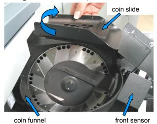
Please fold up the coin tray unit and beginn the cleaning with the enclosed scraper.
