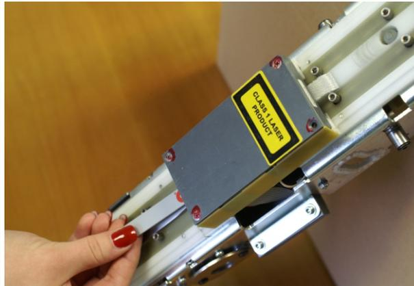
Attention: While insertion the cleaning pad has to face upwards!
